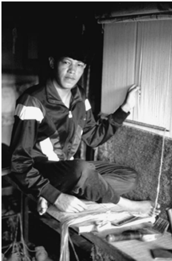
FIGURE 1 Contemporary Tibetan upright loom showing the steel rod used to make the pile. The carpet is of an 'open field' design, for export to Germany
